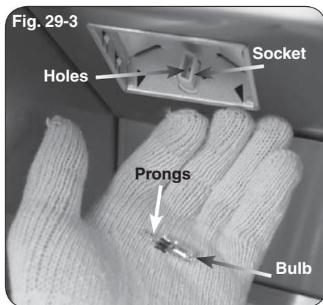
7. Insert the new **12V / 10 watt** halogen bulb into the socket so that both pins slide all the way into the two holes in the bottom of the socket.
