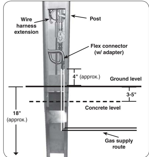
**Fig. 14-2** In-ground install orientation
