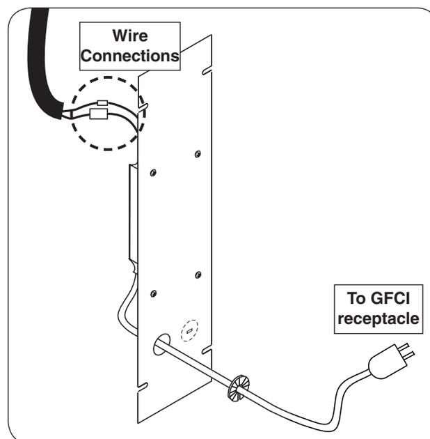
Fig. 16-2 Connect: Wires, Plate, Power
