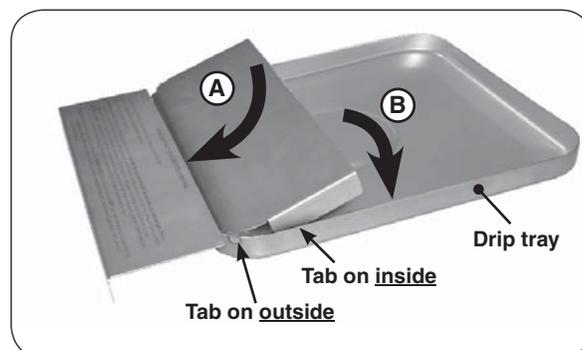
**Fig. 27-2** Install drip tray heat shield
