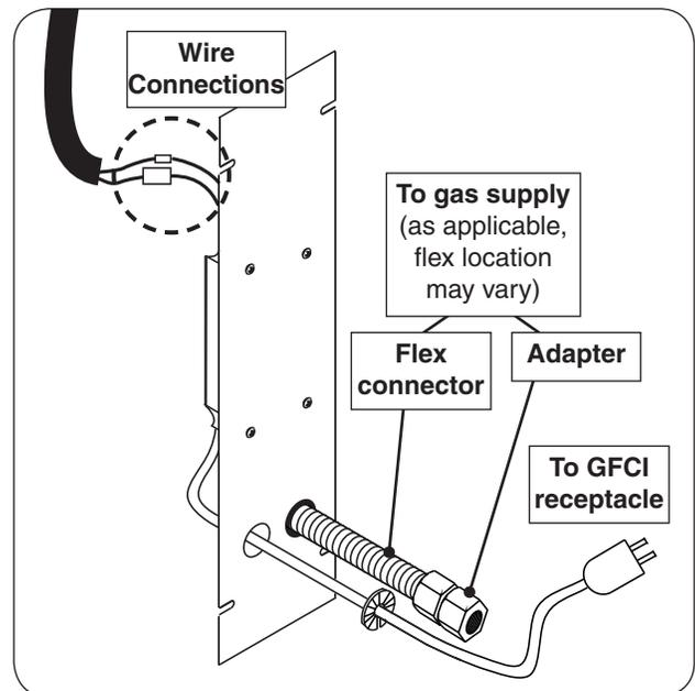
Fig. 13-1 Connect: Gas, Wires, Plate, Power
