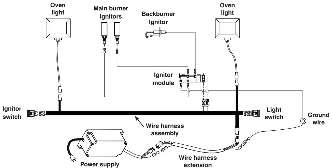
\* Backburner model shown. Model wire diagrams may vary.
