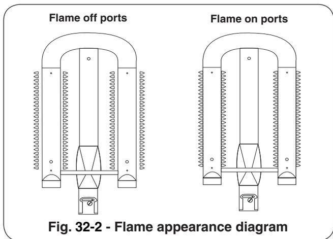
Fig. 32-2 - Flame appearance diagram
