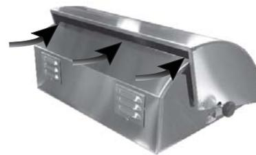
YOU MUST PROTECT REAR OVEN VENT FROM PREVAILING WIND
