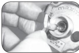
**STEP 4:** Replace the unit into the regulator and screw down until snug.
