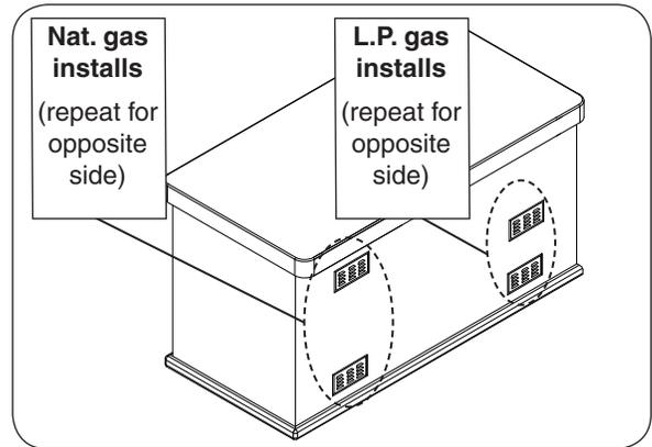
Fig. 12-1 Ventilation detail
