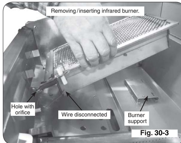
4. Using a  $\frac{1}{2}$ " deep socket, remove the orifice from the valve. Access this through the hole in the forward firebox plate (see PARTS LIST and Fig. 30-3).
