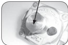
**Note:** Each end of the plastic converter is engraved with either the letters "NAT" or "L.P." (propane) for the respective gasses. When the converter is in the cap and the cap is held uppermost, the letters seen indicate the gas that the regulator is set up for.
