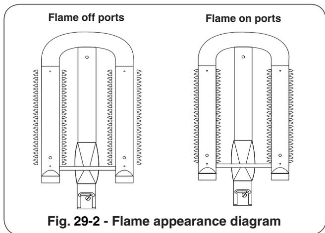
the air shutter until the flames appear to burn while touching the burner ports (Fig. 29-2). If flames are a lazy yellow, open the air shutters until the flame is mostly blue.
