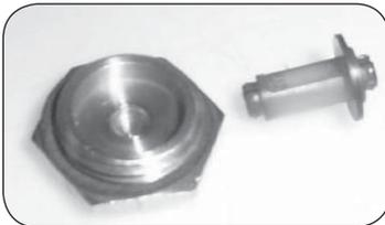
**STEP 2:** Remove the converter (the plastic stalk) by carefully pulling it away from the center of the cap (it will snap out of its seating).
