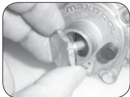
**STEP 1:** Unscrew and remove the cap from the regulator, extracting the converter.
