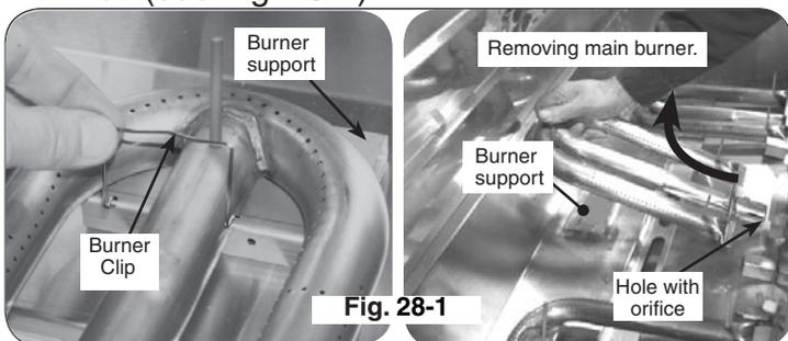
3. Using a 1/2" deep socket nut driver, remove the orifice from the valve. Access this through the hole in the forward firebox plate inside the grill (see PARTS LIST and Fig. 28-1).
