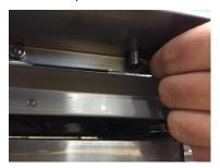
3. Remove the crossfire panel. The crossfire panel is a downward U shaped channel located between the burners towards the rear of the burners. The crossfire panel is removed by unscrewing the fastener under the channel which holds it in place. The most commonly used fastener can be removed with a metric #4 Allen wrench included with the sear burner.
