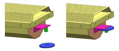
5. With either of the above configurations, replace the cotter pin to hold the burner firmly in place if you
