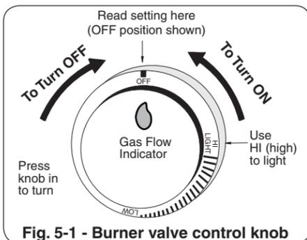
Fig. 5-1 - Burner valve control knob
