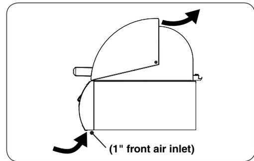
Fig. 10-1 Airflow diagram
