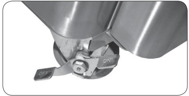
Fig. 20-1 Lock/unlock wheels
