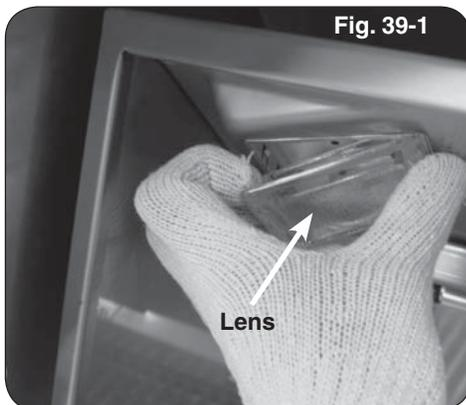
5. Wearing a pair of gloves, reach into the fixture, gently grab the bulb, and pull it straight out of the fixture so that the two pins at the base of the bulb come all the way out.
