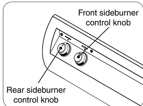
**Fig. 24-3 Double sideburner controls**
