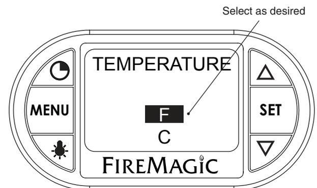
Fig. 30-3 Temperature scale screen
