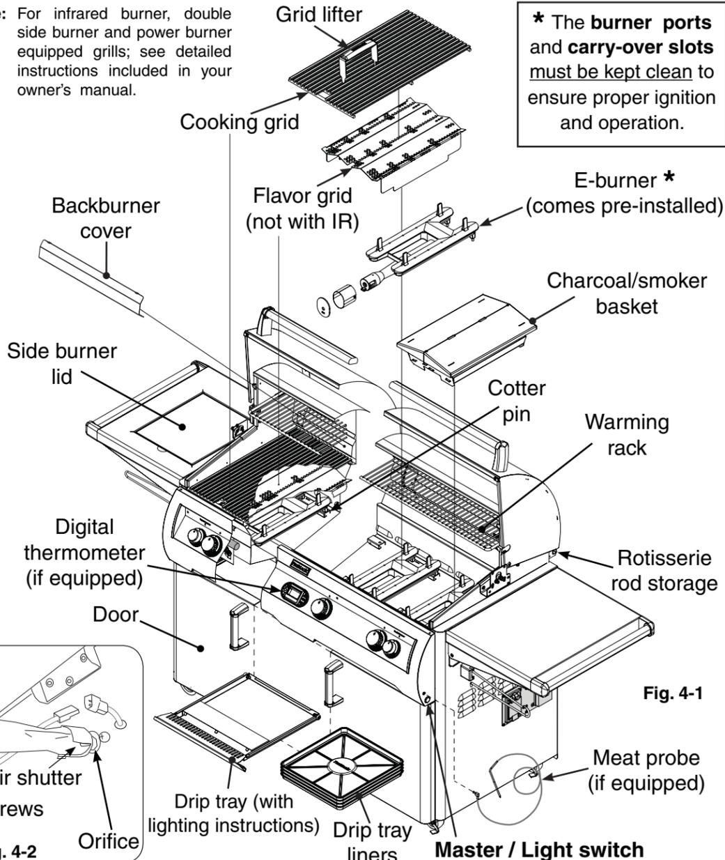
**\* The burner ports and carry-over slots must be kept clean to ensure proper ignition and operation.**
